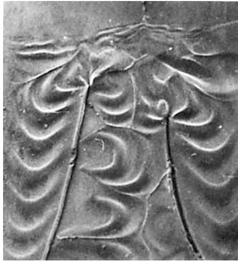
Fig. 11. Fracture surface of specimen cycled at 10^{-1} Hz in methanol.
